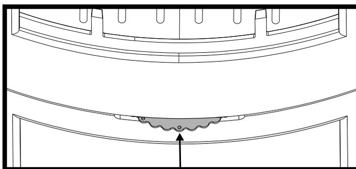
**Position fermée du registre d'arrivée d'air**
